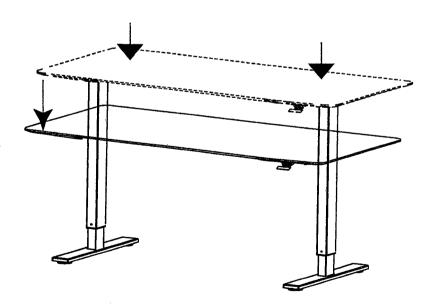
Lift the paddle and push the table down to lower the height.
